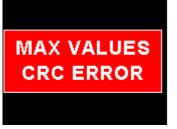
Max Values CRC error. Load default settings to restore to factory defaults. If the error message still persists then it could possibly be a non-volatile memory failure in which case the instrument will then have to be returned to the factory.
